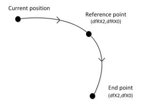
Description Moves from current position, through indicated reference point to the end
