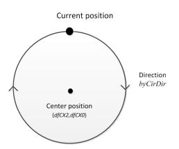
Description Moves in a complete circular trajectory around the indicated center in the
