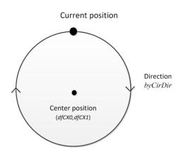
Description Moves in a complete circular trajectory around the indicated center in the
